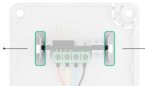
3. Prepare holes for cable output in advance. To output cables from the back of the keypad, break out the perforated part on the SmartBracket mounting panel. To output cables from the bottom of the keypad, make holes in the bottom of the enclosure using a drill bit, a special milling cutter for small holes, or hand-cutting tools.
