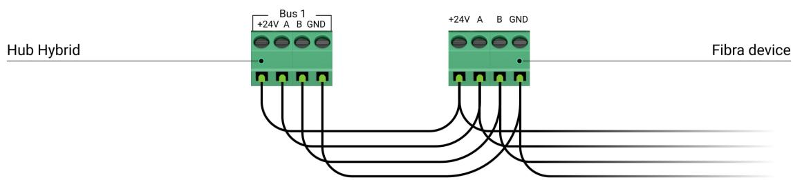
For the **Beam (Radial)** topology, be sure to install a 120 Ohm terminating resistor at the end of the line (included in the hub complete set). The terminating resistor is connected to the signal terminals of the last detector on the line.
