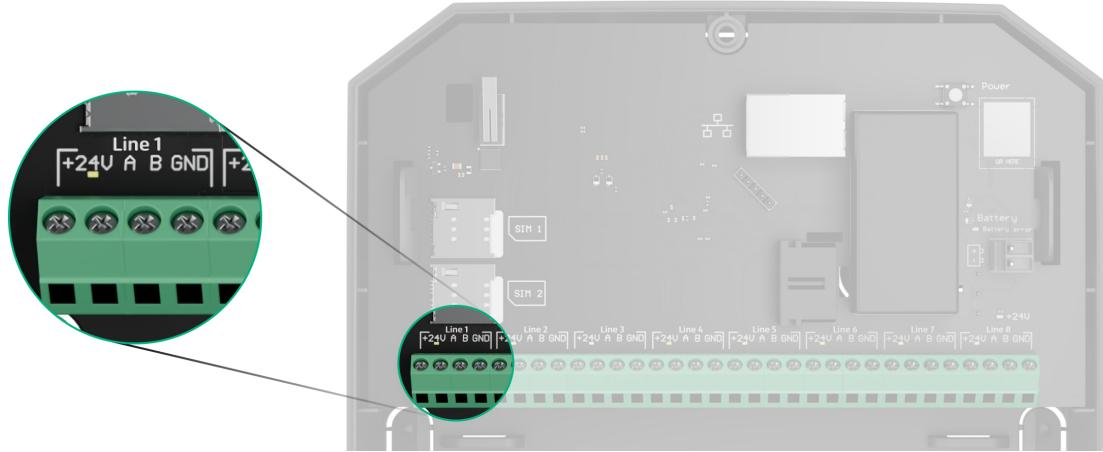
**+24V** – power supply terminal of 24 V $_{\text{--}}$ .
