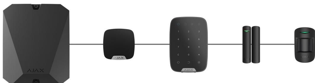
**Ring connection method** occupies two Fibra lines of the hub. If the ring breaks in one place, no device will be disabled. The ring reconfigures into two lines,
