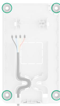
9. Install the KeyPad Fibra board on special mounting panel holders.
