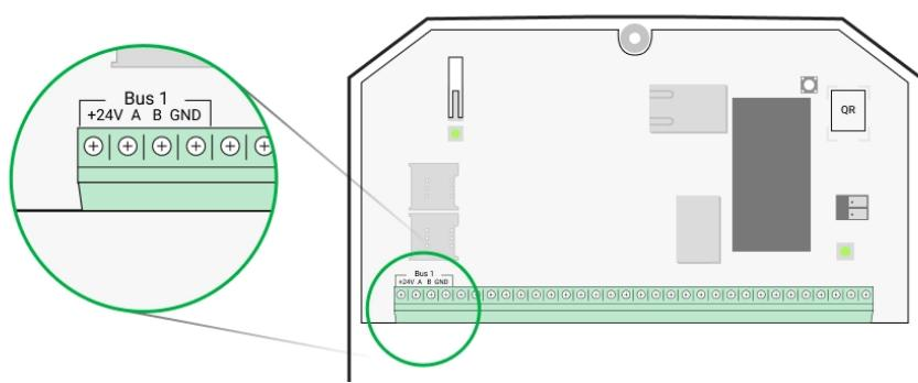
**+24V** – power supply terminal of 24 V $_{\text{--}}$ .
