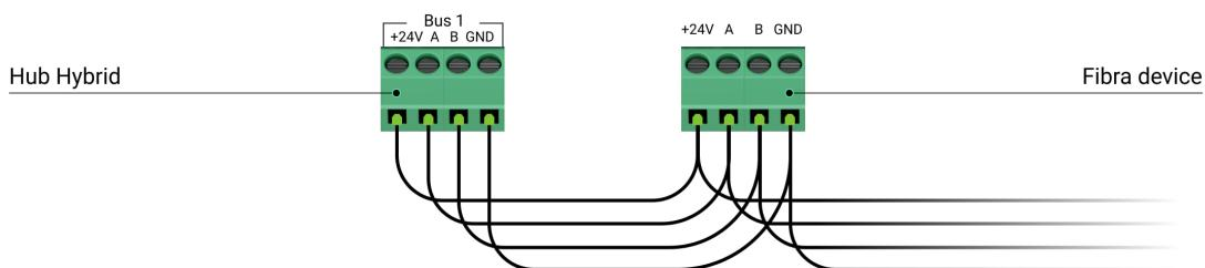
**+24V** – power supply terminal of 24 V $_{\text{--}}$ .
