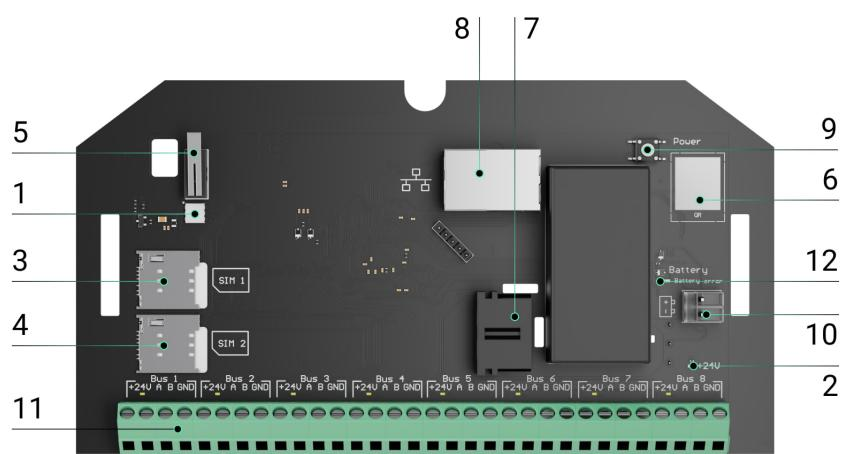
1. LED status indicator of the hub and connected communication channels.
